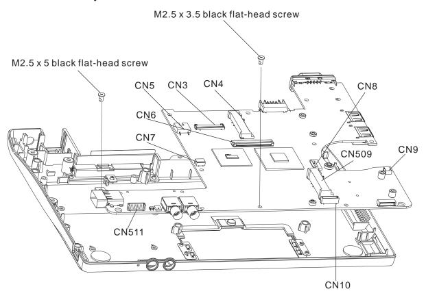
Figure 4-16 Removing the system board
